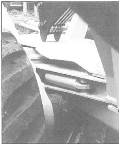
Lenkbarer Bogie am Rottne Rapid Forwarder
